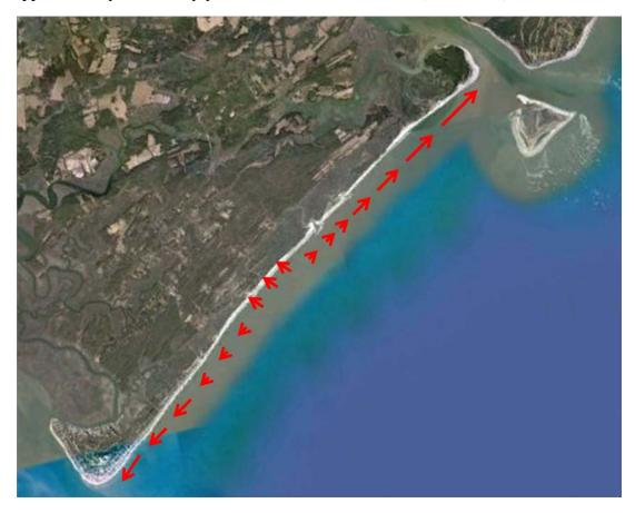
Figure 2: Longshore sand transport regime between North Edisto Inlet and South Edisto Inlet.
