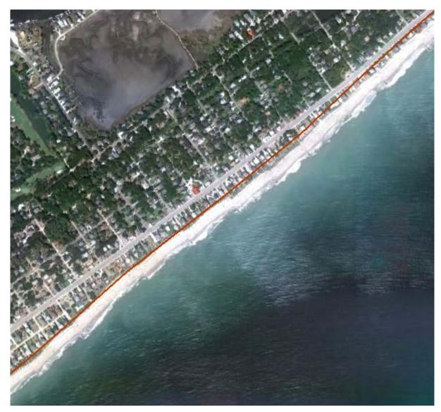
Figure 39: Without-project forecast of average shoreline position in 2064 between groin cells 12 and 20.
