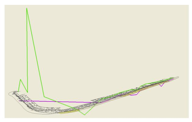
Figure 34: Three dimensional representation of MHW shoreline change rates (ft/yr) for OCRM beach profiles along Edisto Island (green represents rates including the 1995 & 2006 nourishments, purple represents rates excluding the 1995 & 2006 nourishments).
