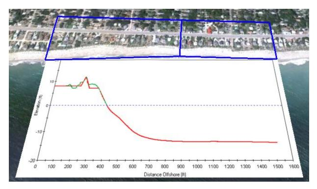
Figure 18: Representative and idealized beach profile for Reaches E4 and E5.
