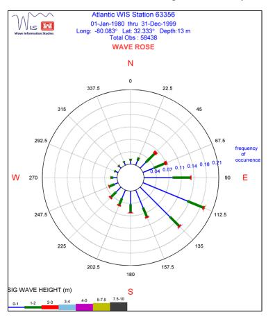
Figure 8- Waverose diagram at WIS station 63356
