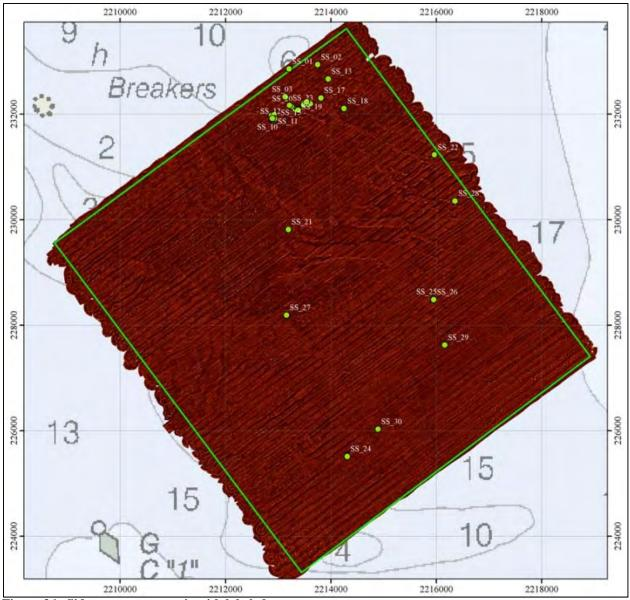
Figure 36. Sidescan sonar mosaic with labeled contacts.
