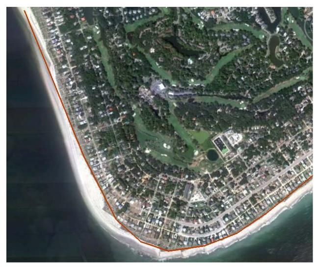
Figure 38: Without-project forecast of average shoreline position in 2064 along the inlet shoreline and around the Point to Groin cell 21.
