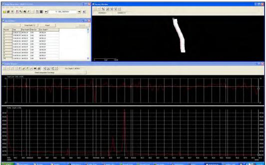
Figure 29. Hypack Single Beam Editor magnetic data display of a section of a survey line. Using these windows one can analyze anomaly position, strength, duration, and type. The peaks of these variations are the locations of target coordinates; their width is the duration.
