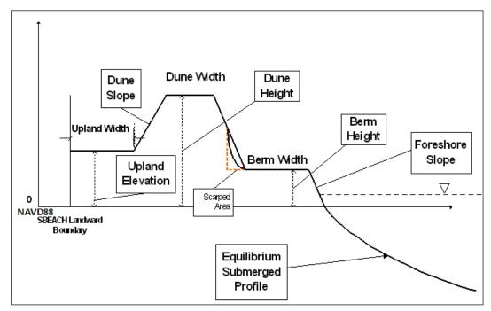
Figure 3.6: Features of an idealized shore profile cross-section.
