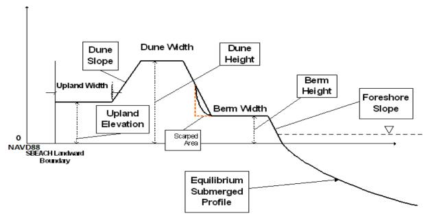
Figure 1.4-2 Shore profile cross-section
