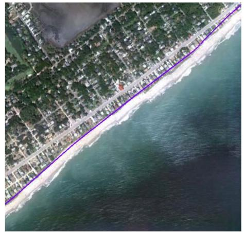
Figure 4.2: Predicted location of the shoreline between reaches E4-E7 (purple line) after 50 years in the future without project scenario.
