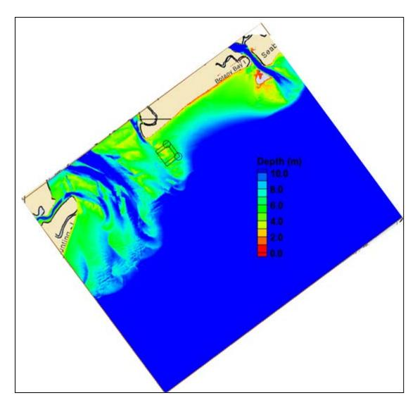
Figure 7- CMS-WAVE grid bathymetry
