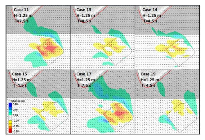
Figure 15- Wave height change for wave condition 11, 13, 14, 15, 17 and 19
