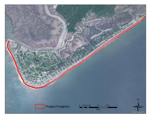
Figure 2. Project footprint from landward toe of dune to seaward berm crest
