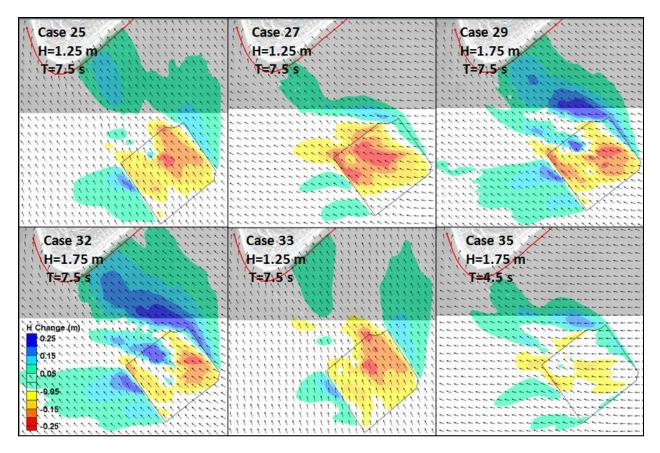
Figure 16- Wave height change for wave condition 25, 27, 29, 32, 33 and 35
