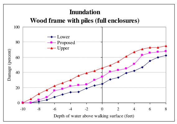
Figure 6.3: Damage functions used to measure erosion damage to fully enclosed structures with piles.
