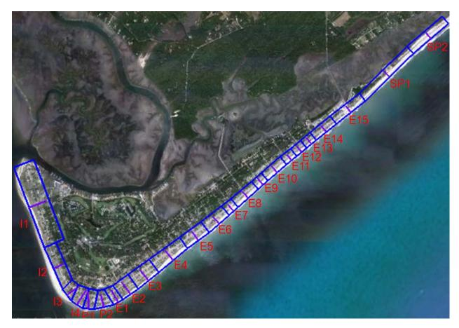
Figure 31: Beach-fx reaches and SBEACH reference lines.
