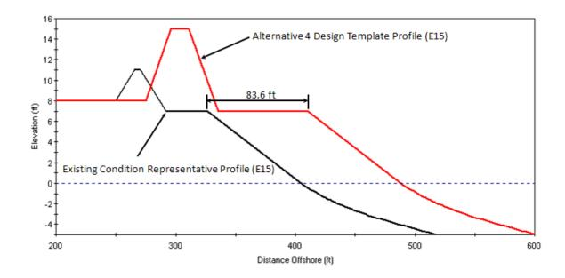
Figure 51: Groin Lengthening Estimation Technique.
