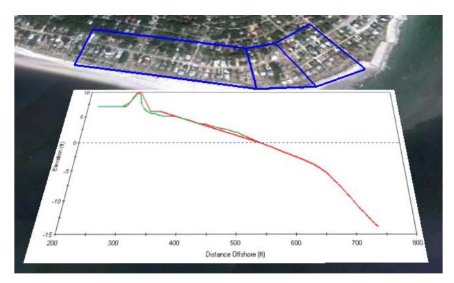
Figure 13: Representative and idealized beach profile for Reaches I2 through I4.
