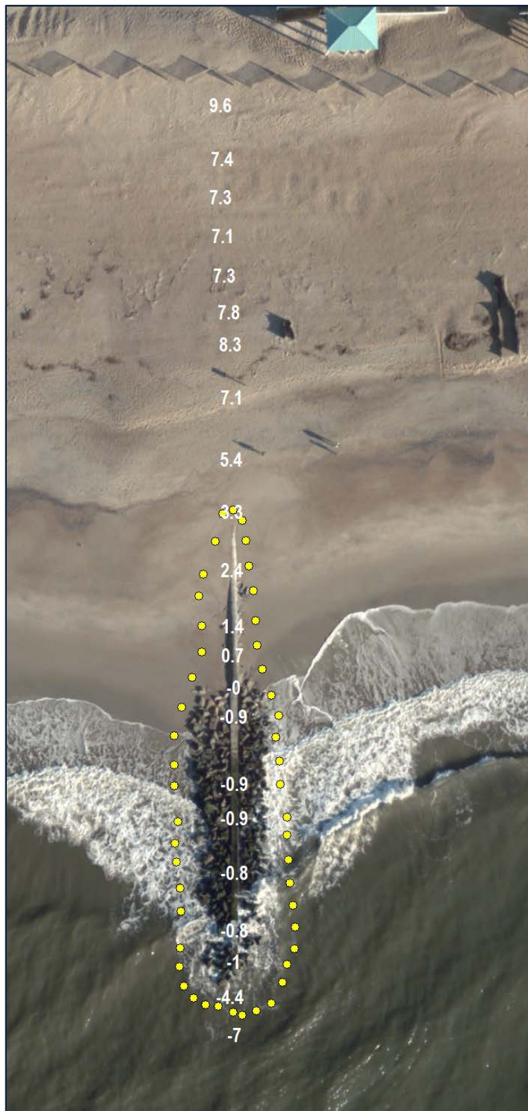
FIGURE 4.6. Plan view of a typical groin extension using sheet pile and concrete cap. Elevations are labeled in white and the footprint of the accessible armor stone is shown in yellow. This extension began near the “0 ft NAVD” contour.
