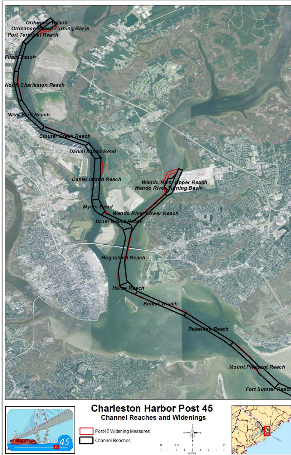
Figure 1-3. Charleston Harbor Channel Reaches and Widenings Source: USACE 2014a
