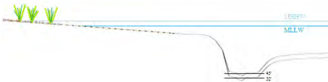
Figure 2.5.16. Crab Bank Cross-section with authorized depth of 45 ft compared to a 7 ft deepened harbor (52 ft depth) at low tide and high tide, neglecting any advance maintenance dredging for simplicity
