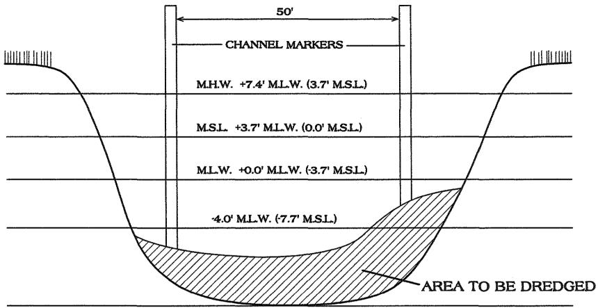
NORMAL WATER DEPTH: -8.0' ML.W. (-11.7' M.S.L.)
