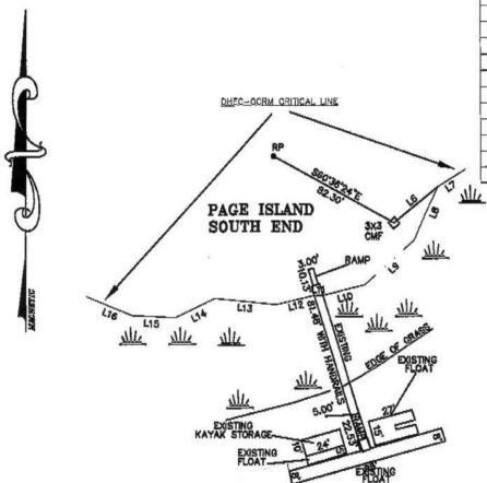
LINE TABLE BEARING LINE LENGTH 33.98 L6 N50°34'55"E L7 19.23 N57'33'37"E L8 21.59 N24'31'45"E N48'06'31"E L9 39.90 25.35 L10 N75'44'16"E L11 6.15 N87"28'44"E 23.04 L12 N76"32'44"E 36.77 L13 S84'01'18"E 26.07 L14 N63'16'33"E L15 25.61 S86"47'40"E L16 29.25 S67'14'48"E
