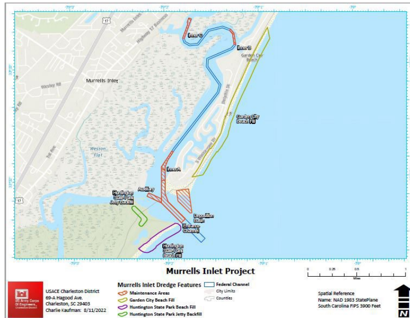
Figure 2-1. Murrells Inlet Federal Navigation Project dredging and material placement footprint (Corps 2022).
