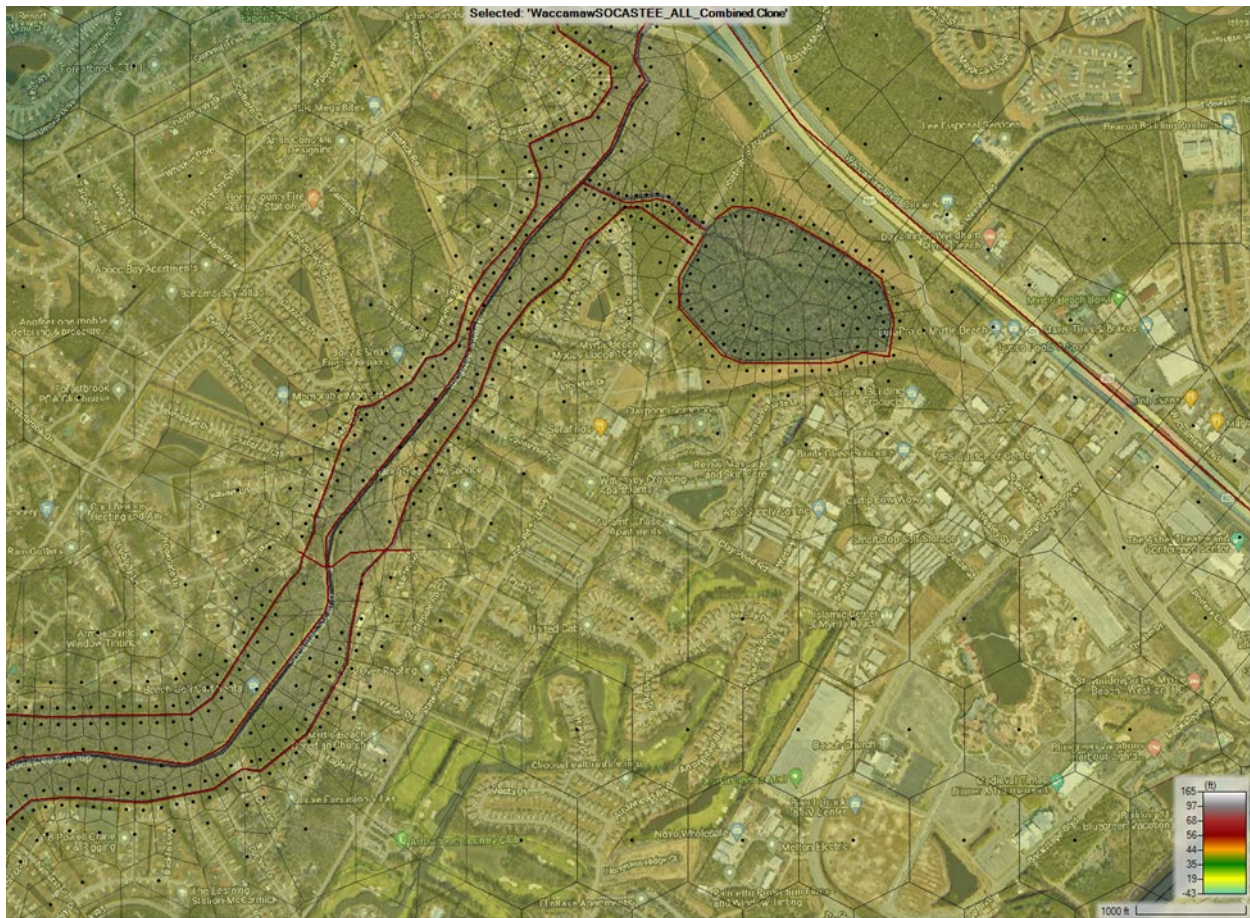
Figure H-21. Refinement of the HEC-RAS grid and topography of the detention pond and channel in Socastee
