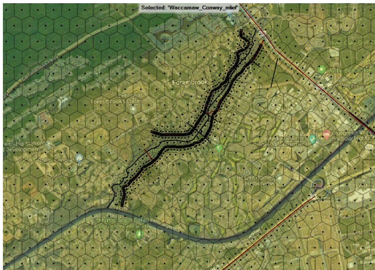
Figure H-20. Evaluated Structural measure of floodwalls along Socastee Creek in Socastee, with grid refinement
