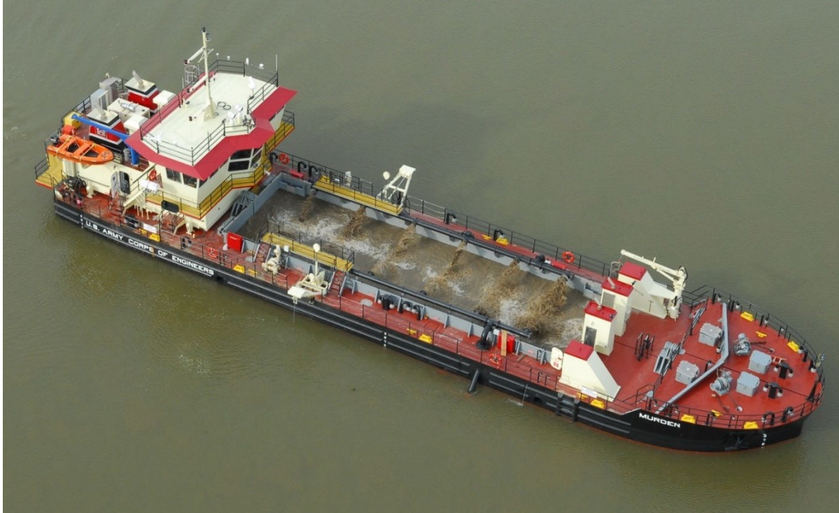
Figure 4. Modified Hopper Dredge, MURDEN dredging the Barnegat Inlet, N.J. in April 2014. Photo by: Tim Boyle
