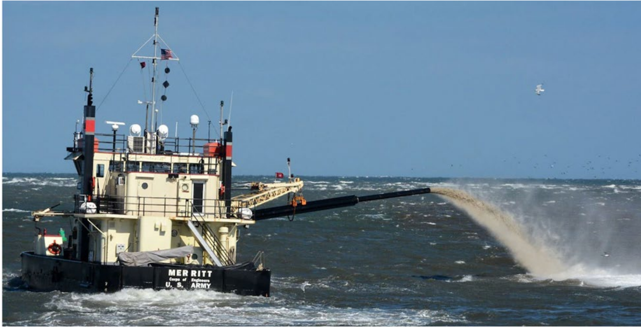
Figure 3. Side-cast Dredge MERRITT at Oregon Inlet. Photo by: Hand Heusinkveld
