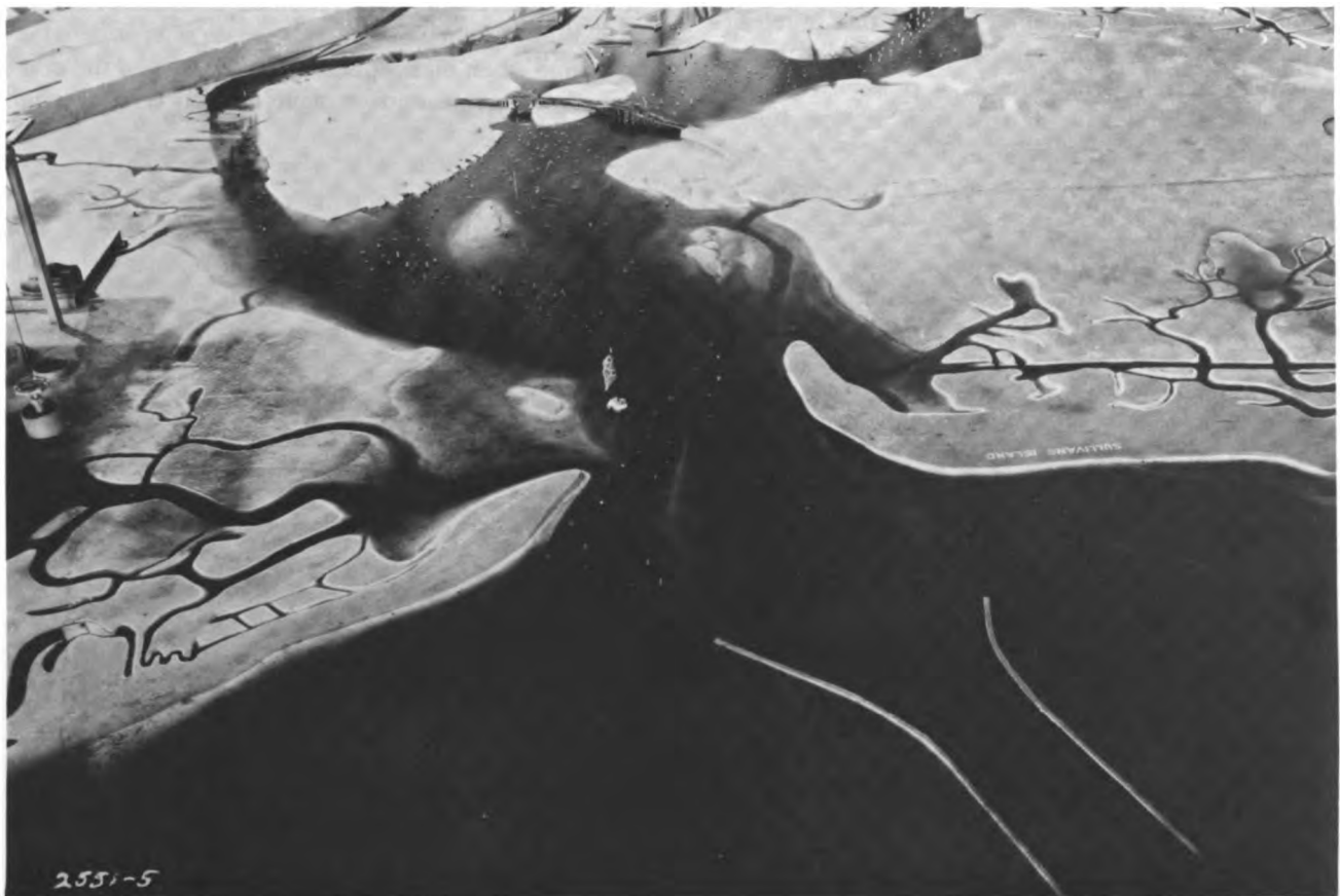
The model of Charleston Harbor constructed by the U.S. Waterways Experimental Station, Vicksburg, Mississippi. Before any plans for reducing the shoaling in Charleston Harbor were made carefully controlled experiments tested alternative solutions.
