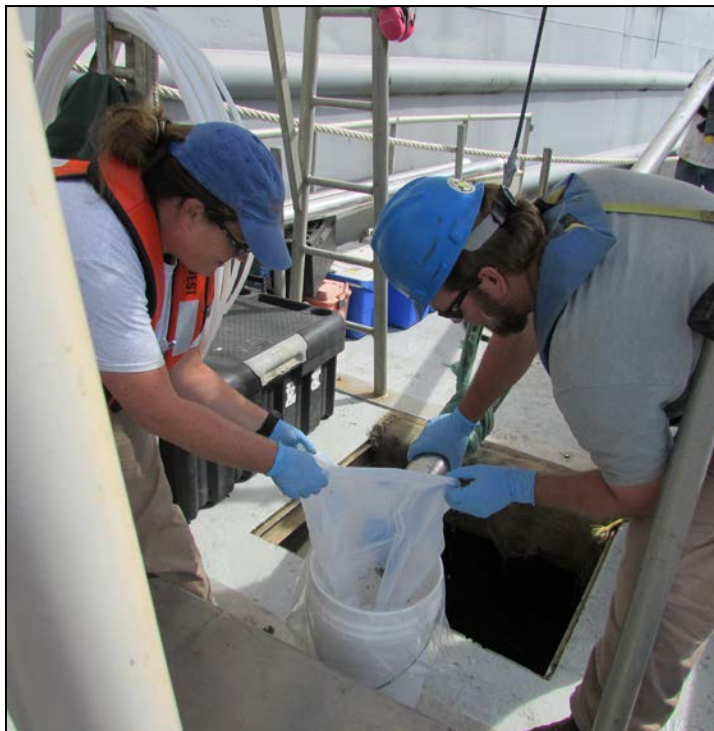
Extruding core sample into decontaminated Teflon® bag
