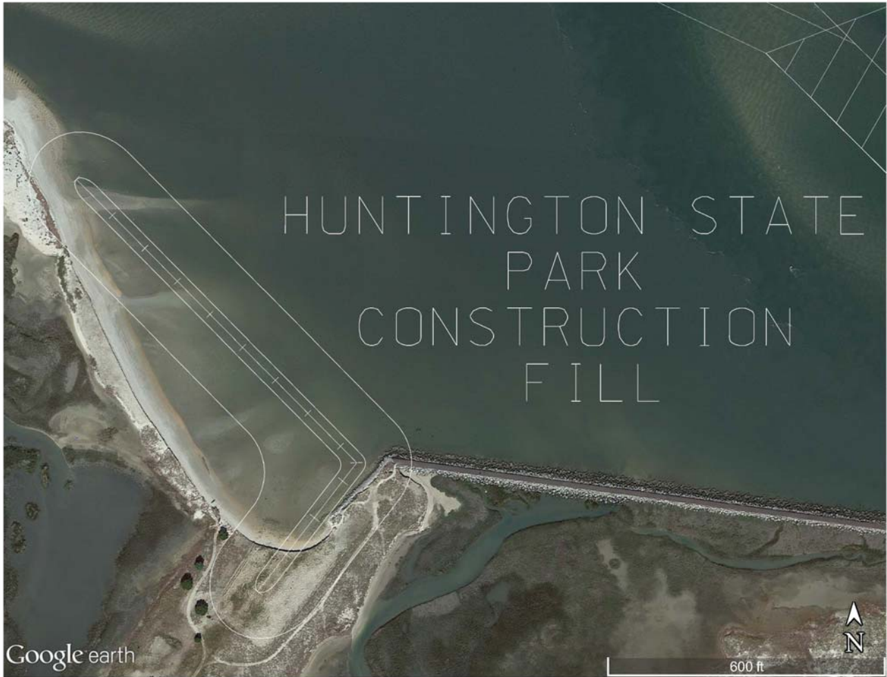
Figure 5. Proposed Depositional Placement Area. The Center Line Indicates Mid-point of Construction Shown in Figure 6
