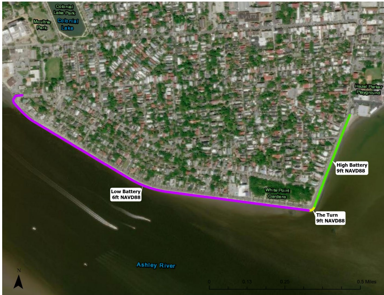
Figure 3-2. The Low Battery Wall is currently being rebuilt and raised to match the elevation of the High Battery Wall.
