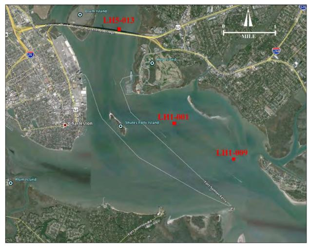
Figure 22. Targets LH1-001 and LH1-009 were located just outside the eastern side of the channel in the lower part of the harbor. However, Target LH5-013 was on the edge of the channel just upriver from the eastern bridge bent of the Ravenel Bridge in the upper harbor. Debris at this latter target was problematic for both anchoring and diver safety (base map courtesy of Google Earth).
