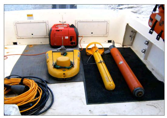
Figure 26. Survey instruments employed during the investigation included (from right to left) the magnetometer, the sidescan sonar, and the subbottom profiler. Honda generator employed to power the instruments is in the background adjacent to the transom.
