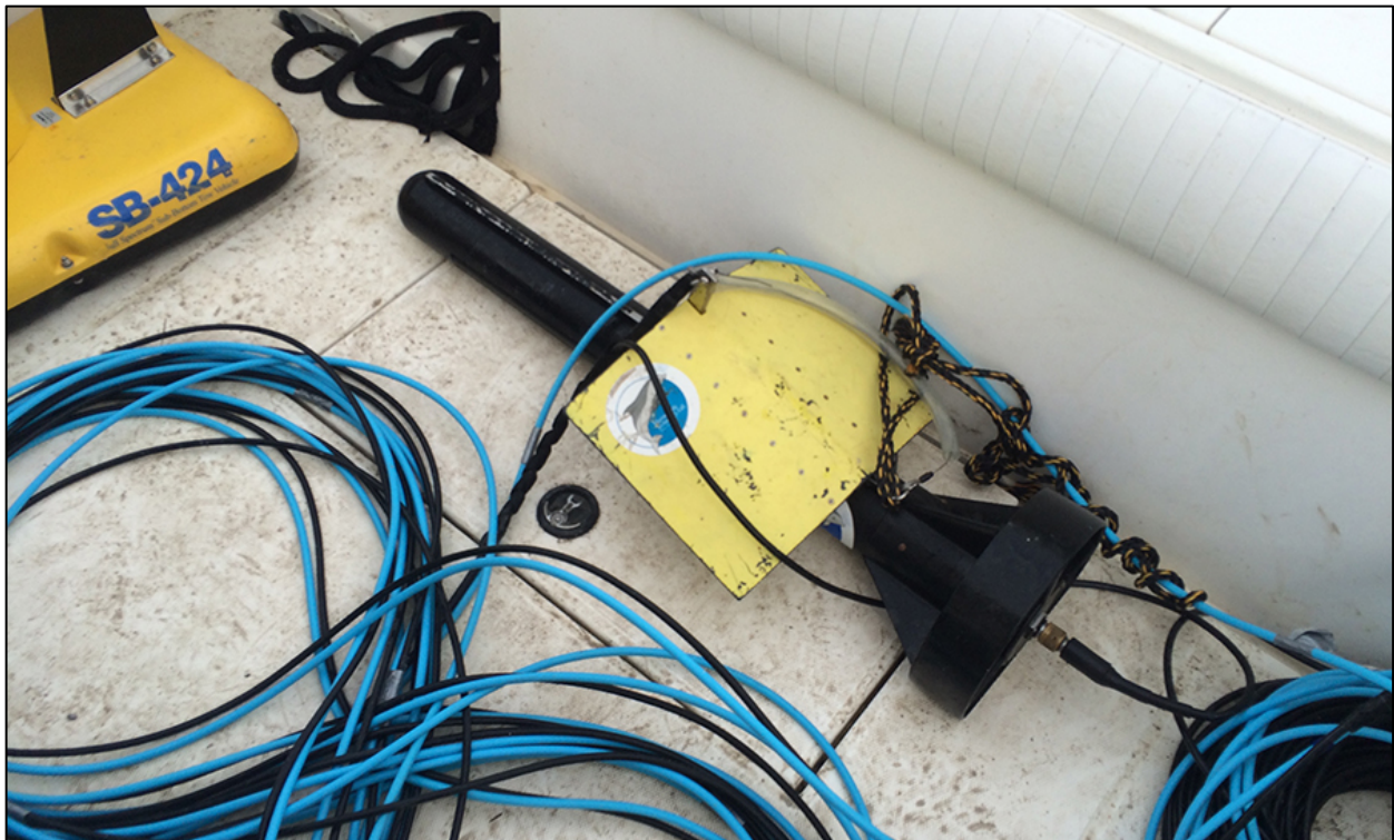
Figure 3-05. Marine Sonic Technology HDS sidescan sonar with 800/900 kilohertz towfish employed during the survey.
