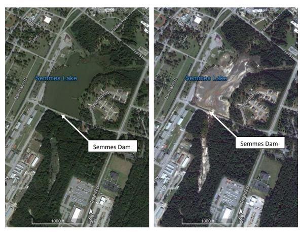
Figure 1.5 - Semmes Lake Before (left) and After Dam Breach (right).
