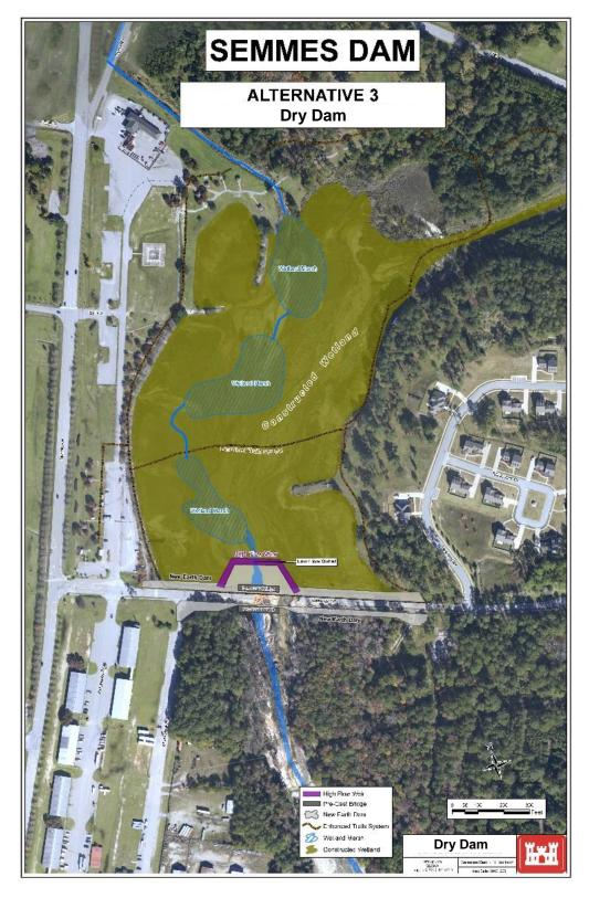
Figure 2.3 - Alternative 3 Rebuild the Dam and Road; Dry Dam (Conceptual Design)
