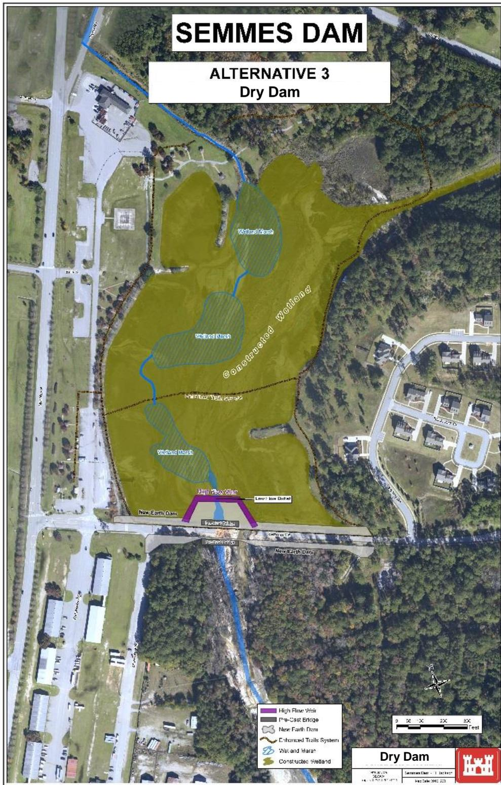
Figure 2.3 - Alternative 3 Rebuild the Dam and Road; Dry Dam (Conceptual Design)
