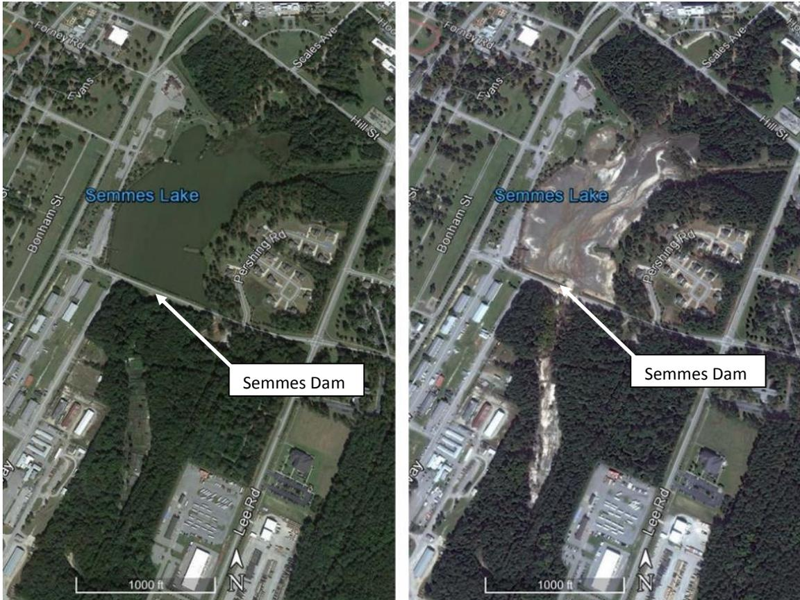
Figure 1.5 - Semmes Lake Before (left) and After Dam Breach (right).
