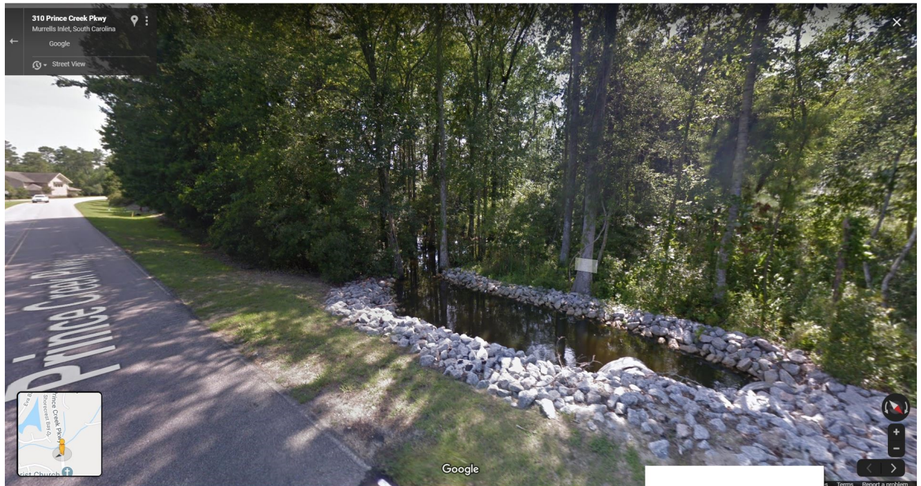
Figure 1: Screen capture from Google Maps street view depicting the direct hydrologic surface connection created by the culvert system when Prince Creek Parkway was originally constructed in wetlands. Photo oriented looking southwest
