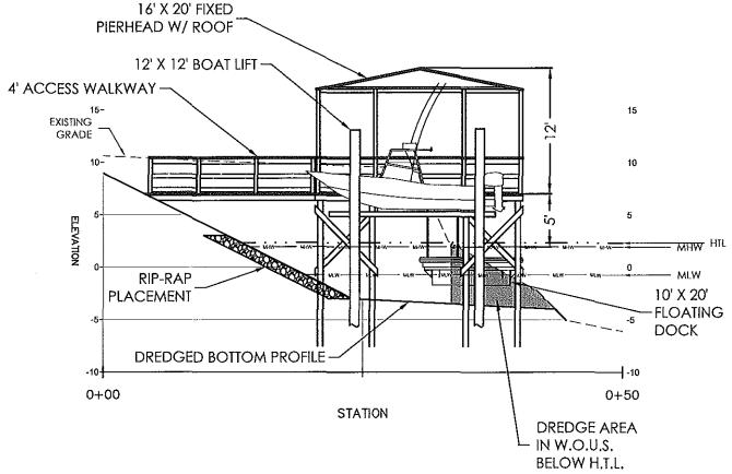
HIGH TIDE LINE (HTL) = +2.323'MEAH HIGH WATER (MHW) = +1.943' MEAN LOW WATER (MLW) = -0.727NAVD88 DATUM
