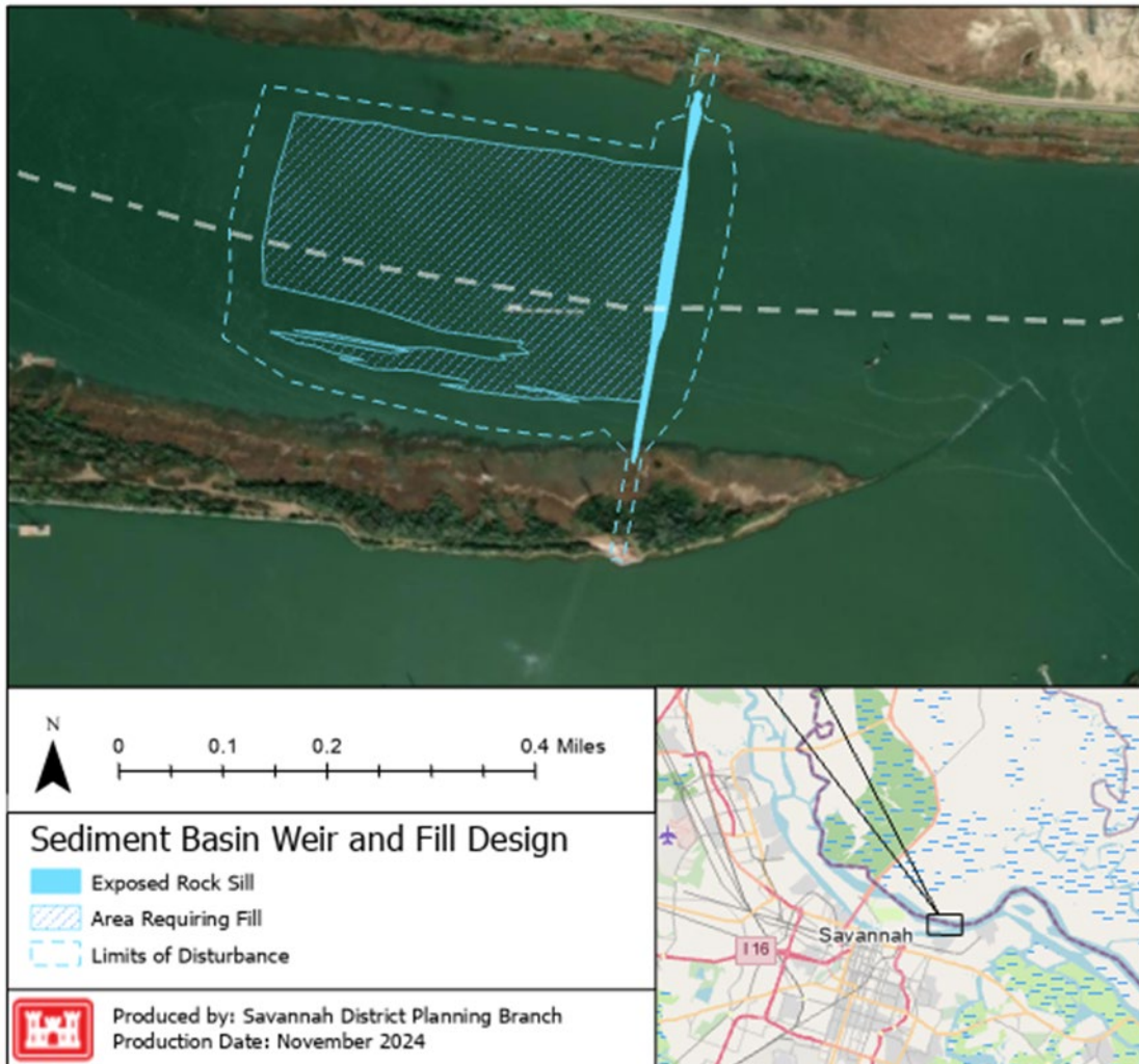
Figure 1. Overview of the location of the sediment basin weir and fill
