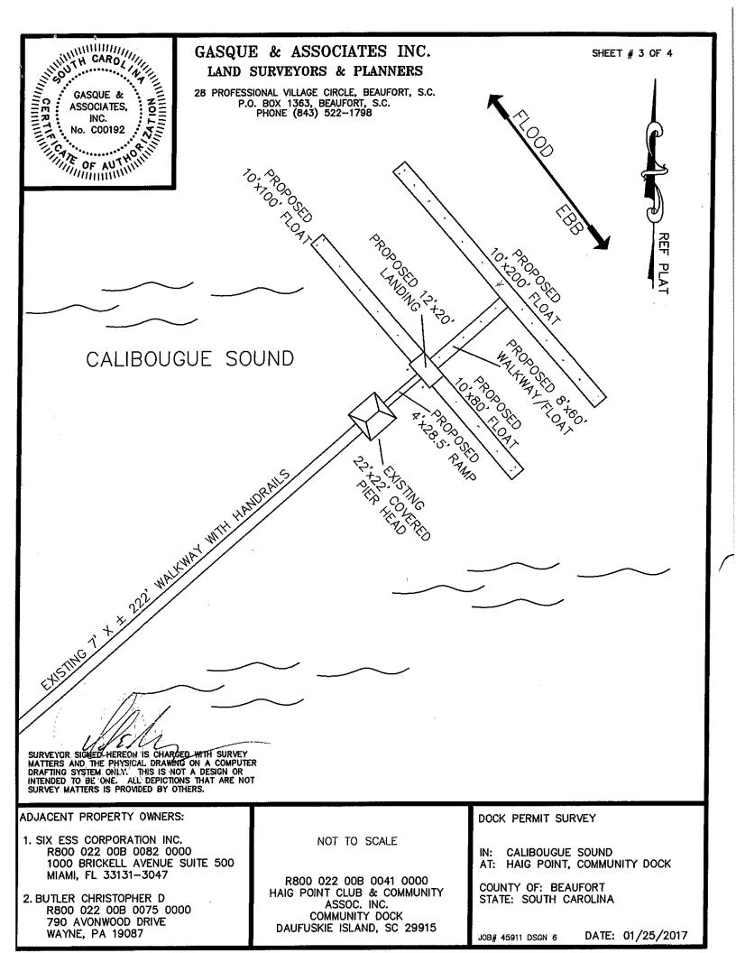
FLOOD EBB TY? PROPOSED G'TYP. 10' × 200' FLOAT PROPOSED 8'x60' WALKWAY / FLOAT PROPOSED 10' × 80' FLOAT PROPOSED 12'X20' 6 Typ. PROPOSED 24 M. Typ. LANDING 4' x28.5' RAMP PROPOSED 10'x100' FLOAT EXISTING 22'X22' COVERED PIER HEAD Proposed Florting Dock PILE LAYOUT PLAN 27ea, 0=12" Ø Timber Rie To be water Jetted & Driven To -20' Bottom of River
