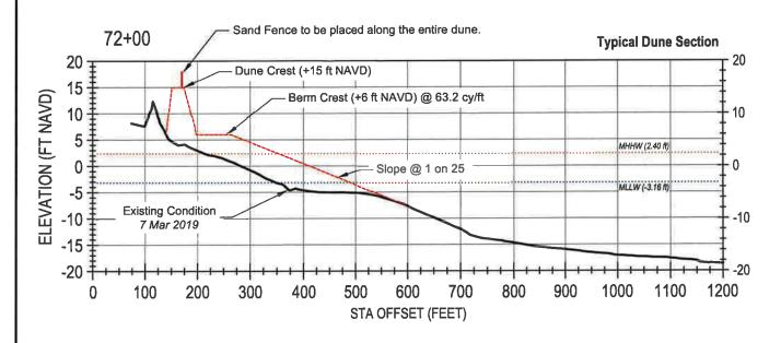
\* Note: Typical profiles shown are the existing condition as of 7 March 2019. Fill volumes may need to be adjusted dependent upon existing conditions at time of construction.
