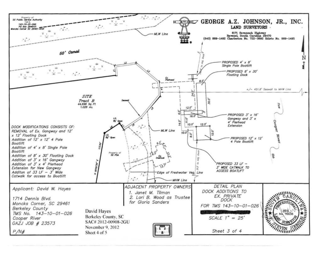
DOCK MODIFICATIONS CONSISTS OF: REMOVAL of Ex. Gangway and 12' x 12' Floating Dock Addition of 12' x 12' 4 Pole Boatlift Addition of 4' x 8' Single Pole Boatlift Addition of 8' x 30' Floating Dock Addition of 3' x 16' Gangway Addition of 3' x 4' Pierhead Extension for New Gangway
